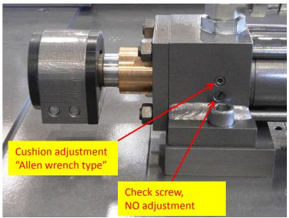
The bottom screw is another internal check, NO adjustment. Use a Allen wrench to adjust the cushion. With the feed drawer installed adjust so the cylinder is NOT binding at end of stroke. This should be check every six months for correct operation.
