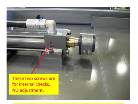
Before installing rod end apply Blue 242 LOCTITE to shaft and pinch bolts threads. Install rear plastic spacer. Thread rod end on till it bottoms out on shoulder and tighten bolts to 125 foot pounds, install front plastic spacer.
